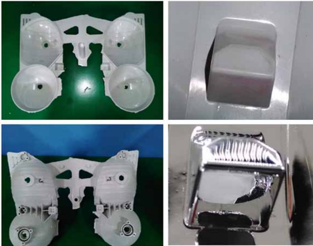
Fig. 5 The actual trial result of the optimized design. There are no air traps observed.
